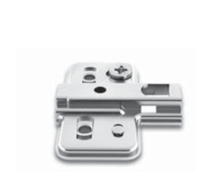
Metal cruciform mounting plate. Selftapping screw fixing. Independent vertical adjustment with CAM. Screws are provided on demand.
