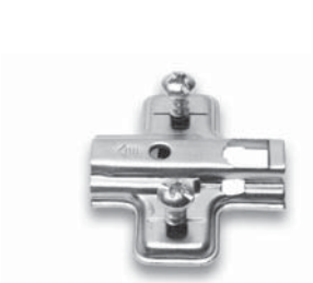
Metal cruciform mounting plate. Premounted selftapping screws Ø4.7mm. Vertical adjustment.
