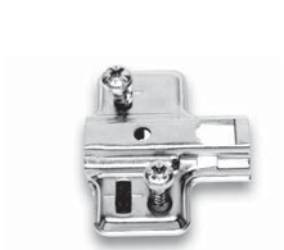
Asymmetric mounting plate for central panel. Fixing by dowels and premounted selftapping screws. Vertical adjustment.
