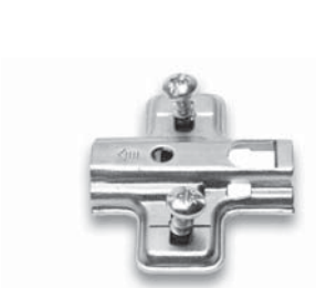
Metal cruciform mounting plate. Fixing by expanding X-Pando dowels Ø5mm. Vertical adjustment.
